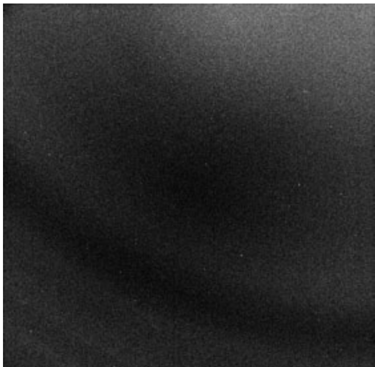
Image 3 is a 60-second dark frame taken immediately after taking another 60-second image of Vega and running the RBIFlush routine before taking the image. The effect of RBI is completely eliminated.
